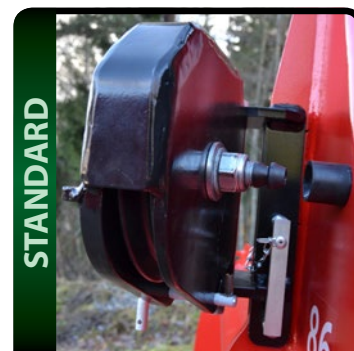
A strong lower pulley can be quick-locked for transportation
